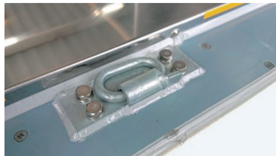
Lashing ring (installed in eight places)
